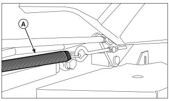
Figure 47. Deck Lift Spring Location A. Deck Lift Spring
